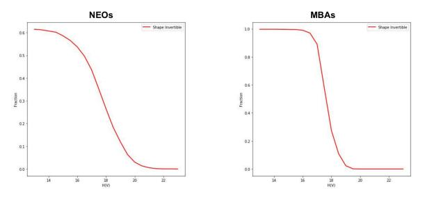
Fraction of LSST detections NEOs and MBAs in the current LSST baseline cadence as a function of absolute magnitude with sufficient numbers of observations to apply light curve inversion techniques to estimate the sizes and shapes of these bodies.
